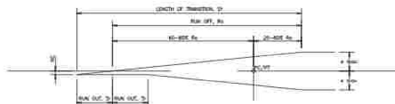
SHOWING HALF OF TRANSITION/EASEMENT - HORIZONTAL CURVATURE AND SUPERELEVATION (DIAGRAMMATIC PROFILE - PAVEMENT REVOLVED ABOUT CENTERLINE)
