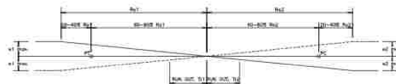
SHOWING HALF OF TRANSITION/EASEMENT - REVERSED HORIZONTAL CURVATURE AND SUPERELEVATION (DIAGRAMMATIC PROFILE - PAVEMENT REVOLVED ABOUT CENTERLINE)
