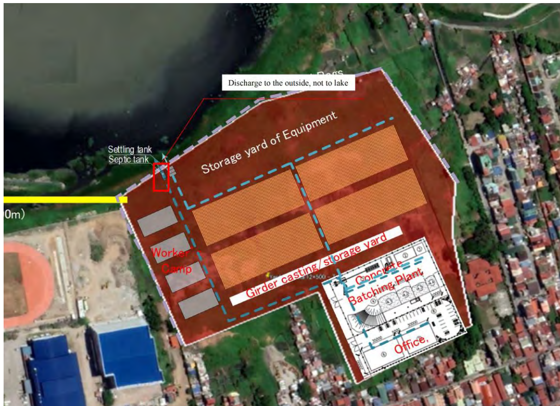
Figure 3-31: Construction Yard for CP2
