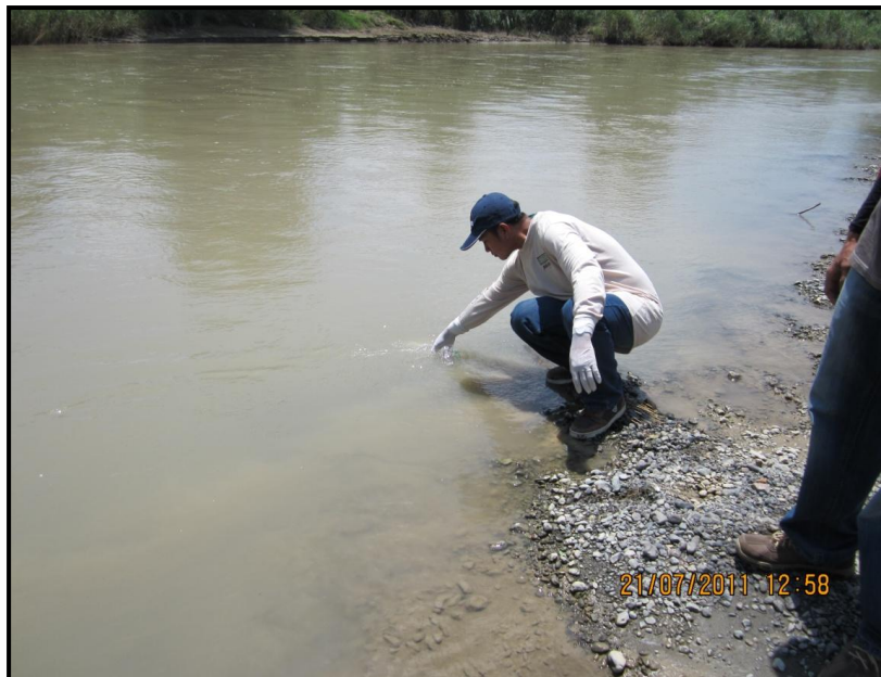
Photo No. 6 Water sample being collected at SSTA.-Talavera River (Upstream)
