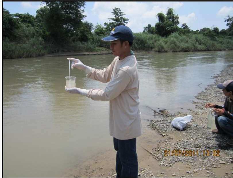
Photo No. 3 Temperature of water sample from the upstream portion of Talavera River was determined using a laboratory thermometer.
