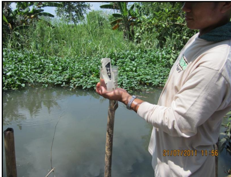
Photo No. 4 On-site measurement of pH of the water sample from San Miguel na Munti Creek was taken using a portable pH meter.
