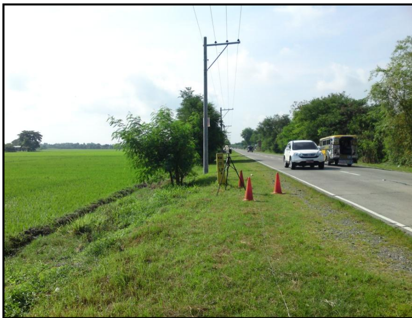
Plate No. 12 Photo showing the TSP level monitoring at Station A2 (Laungcupang)
