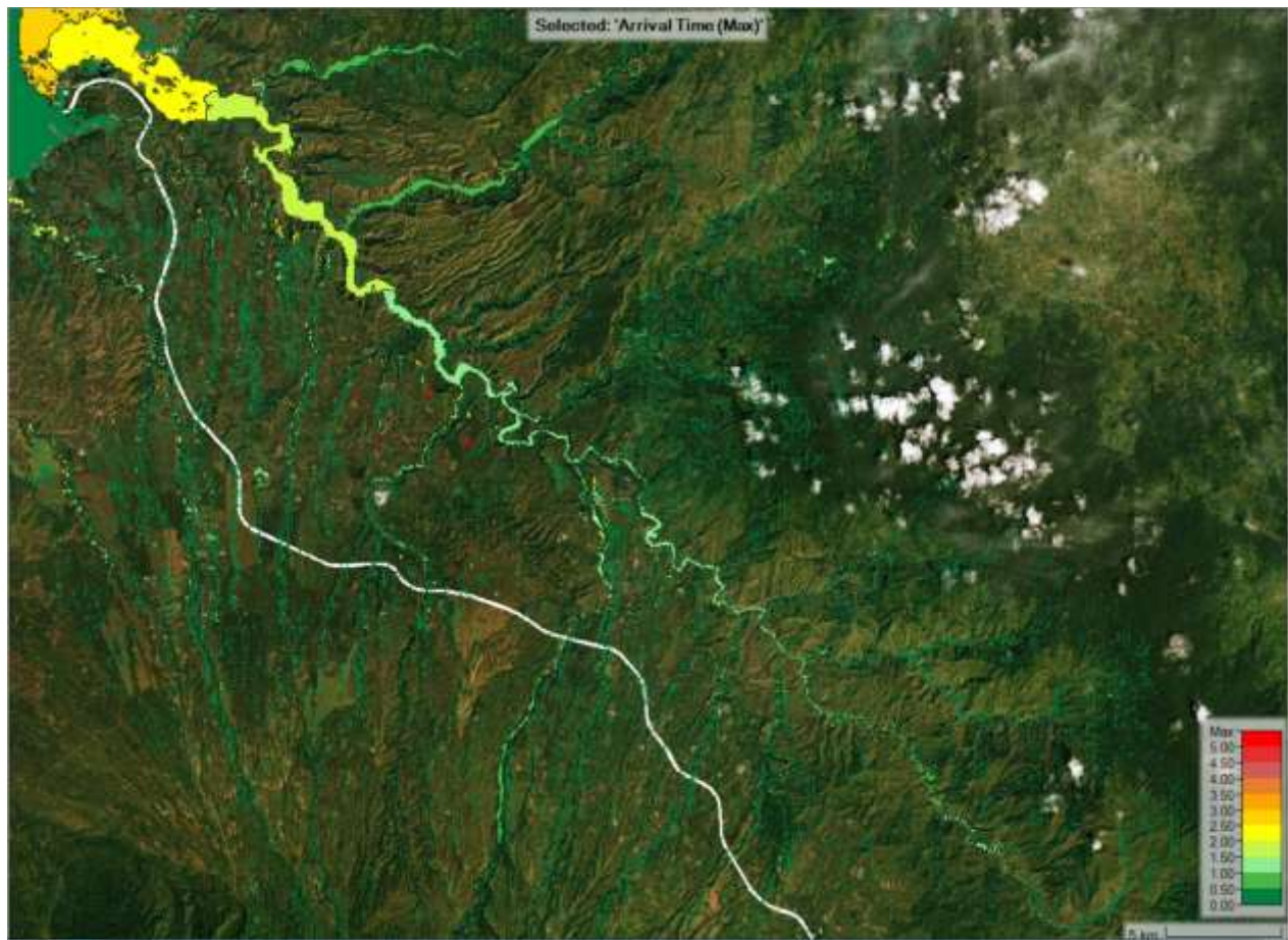
Figure 3-53. Estimated arrival times (hr) of flood peaks as it flows downstream for a 100-year storm event
