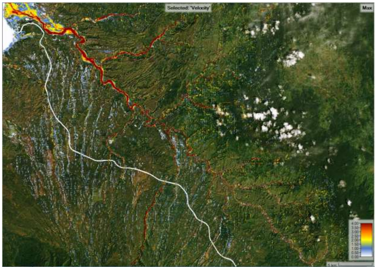
Figure 3-54. Predicted maximum flood velocity map for a 100-year storm event
