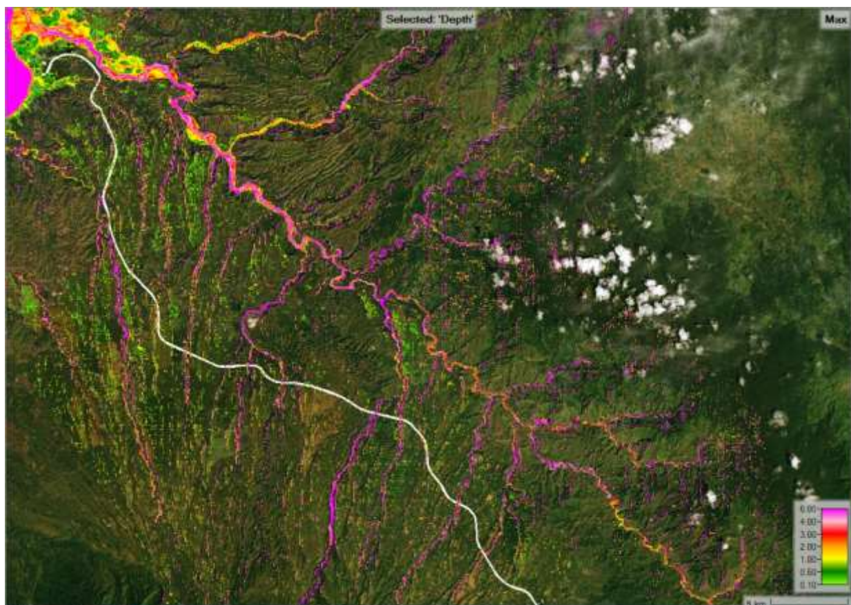
Figure 3-51. Predicted 100-year flood inundation map of the Project site at baseline conditions
