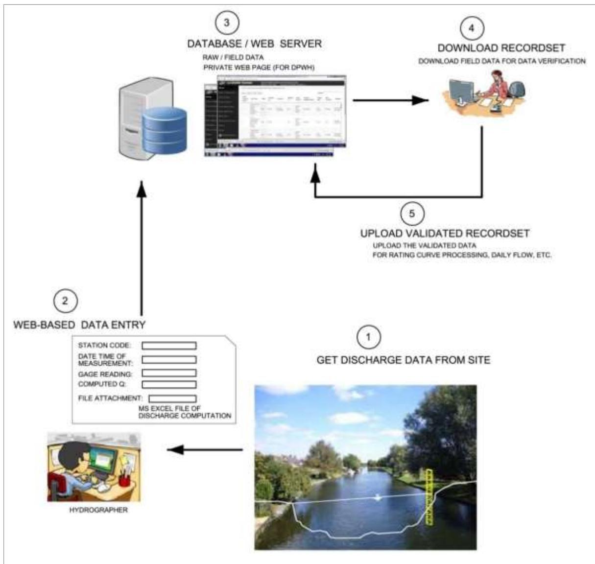
**Figure 6-11. Data flow for Discharge Measurement Collection**
