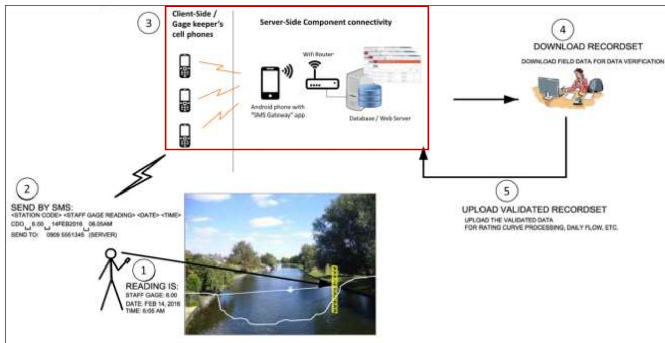
Figure 6-1. Data flow for Water Level Data Collection
