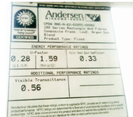
FIGURE 23: Window performance label showing results of SHGC and VLT
