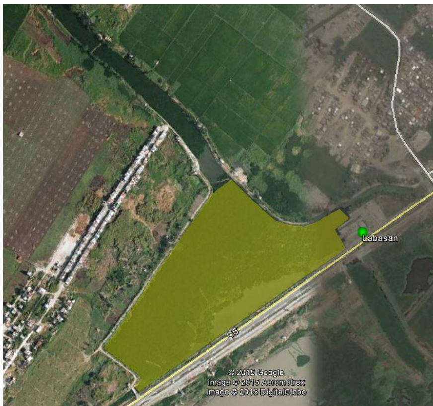
FIGURE 6: LABASAN PS SHOWING THE 6.4 HA STORM ATTENUATION POND. UPSTREAM WATERWAY REMAINS WIDE AND BANKS UNDEVELOPED
