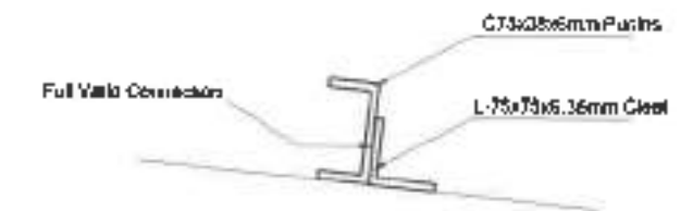
6 PURLINS CLEAT DETAILS S-09 SCALE: NTS
