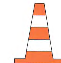
NOTES: 1. TRAFFIC CONES SHALL BE AT LEAST 300MM HIGH OVERALL AND AT LEAST 150MM WIDE AT THE BASE OF THE CONE. THEY SHALL BE FLUORESCENT RED-ORANGE WHEN USED AT NIGHT A MINIMUM OF ONE-THIRD OF THE SURFACE AREA VISIBLE TO APPROACHING TRAFFIC SHALL BE COVERED WITH YELLOW REFLECTIVE MATERIAL. 2. FRAGMENT SHALL BE PROVIDED AT ALL TIMES DURING CONSTRUCTION OPERATIONS. 3. THE CONTRACTOR SHALL ALWAYS MAINTAIN A GOOD CONDITION TRAFFIC CONES. ANY DAMAGED SHALL BE REPLACE WITH NEW ONE.
