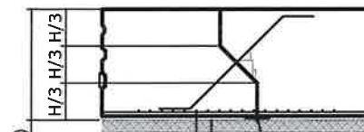
COLUMN VERTICAL BARS EMBEDMENT TO FOOTING DETAIL
