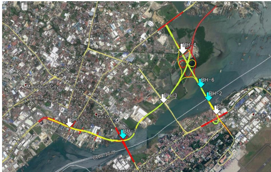
Figure 4.1.19 Google Map Showing the Location of the Seven (7) Bore Holes Drilled by Advanced Geotechnical Engineering Services (AGES) for the 4 th Mactan Bridge Project
