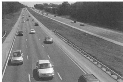
LOS D The level at which speeds begin to decline with increasing flows, with density increasing more quickly.
