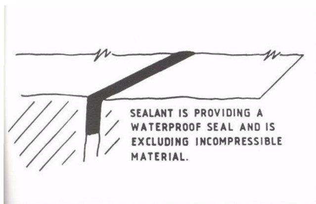
Sealed Joint - Good Condition
