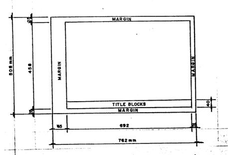
STANDARD SIZE (508 mm X 762 mm). FOR ARCHITECTURAL, STRUCTURAL & MECHANICAL - ELECTRICAL PLANS FOR BUILDINGS PROJECTS
