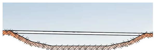
Figure 99. – Adopting the natural landform as a base of ramp
