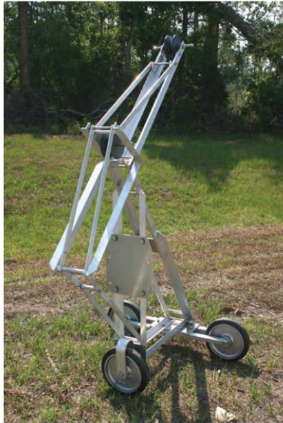
Figure 6-5. Type A crane mounted on a three-wheel base
