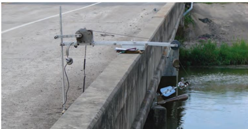
Figure 6-6. Discharge Measurement from a bridge using a bridge board
