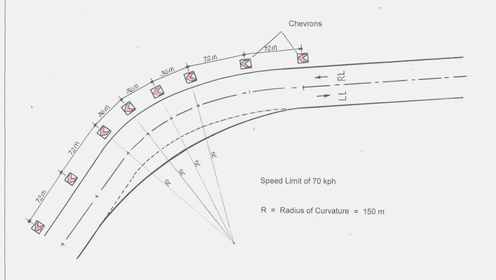
FIGURE 3 - The recommended spacing distances for the Chevron Signs within the curve and approach/departure of the road as shown in Table 620.1 – Recommended spacing for Chevron Signs and as contained in the 6<sup>th</sup> paragraph of Section 620.2.2, Design for Item 620 – Chevron Signs
