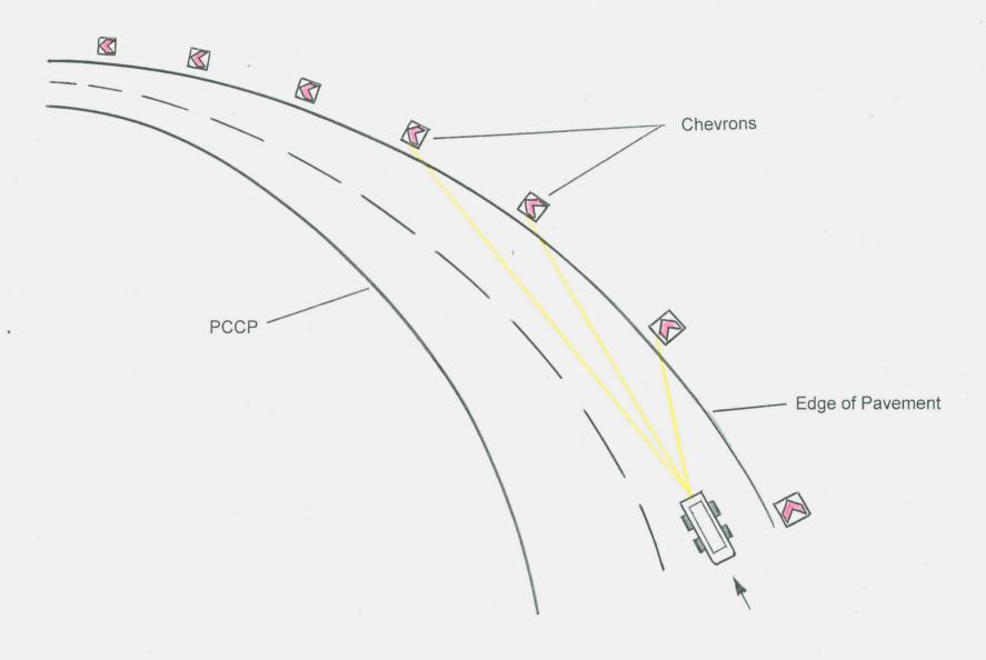
FIGURE 2 - Showing that the spacing of the Chevron Signs allow the driver to see at least three (3) signs in view while negotiating the curve until the change in alignment eliminates the need for the signs as contained in the 4<sup>th</sup> paragraph of Section 620.2.2, Design for Item 620 – Chevron Signs
