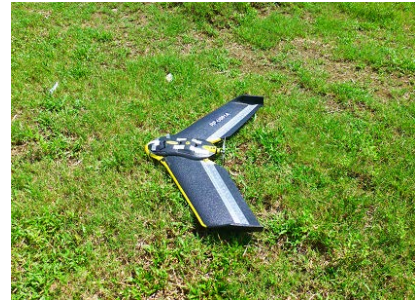
Drone used during Condition inspection of Special Bridge (Fixed Wing type drones)
