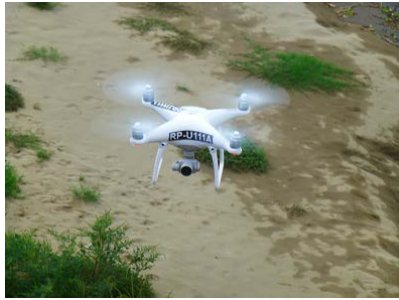
Drone used during Condition inspection of Special Bridge (Rotary type drones)
